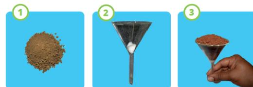
Take 100 ml of air dry soil. Take a funnel and close the neck of the funnel with a little cotton. Put the soil sample on the funnel and gently tap it to make it compact as in natural field condition.
