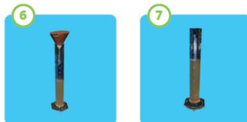
After pouring all the 100 ml water, wait for one hour for the last drop of excess water to drain into the cylinder. Measure the drained water using a measuring cylinder.
