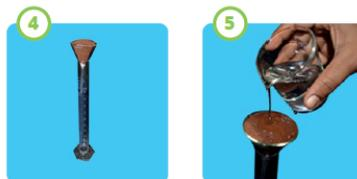
Place the funnel with soil on the measuring cylinder and gently pour 100 ml of water on the soil.
