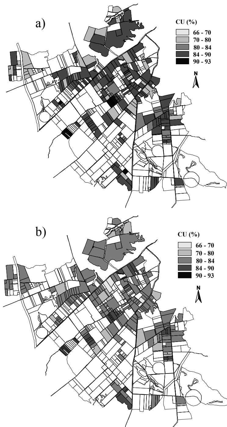
Figure II.4. Spatial distribution of simulated CU in the LQD solid-set plots for an operating pressure of 300 kPa and wind speeds of 1 \text{ m s}^{-1} (a) and 3 \text{ m s}^{-1} (b). Plots in white colour correspond to irrigation machines.
