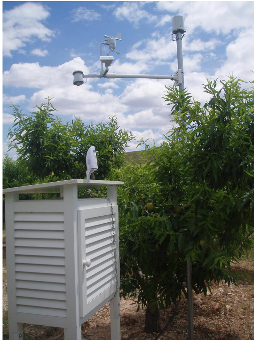
Picture 5.2. Automatic weather station placed within the experimental orchard (Own source).
