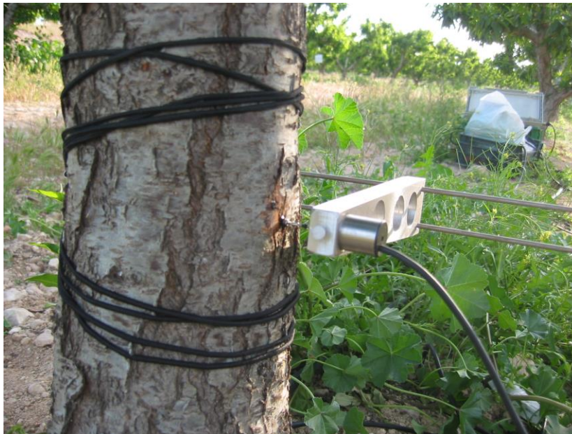
Picture 6.2. LVDT sensor installed in peach “Catherine” (Own source).
